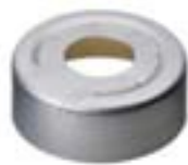
Headspace cap clear lacquered, scorelines break open at 3.0 ± 0.5 bar for pressure release
