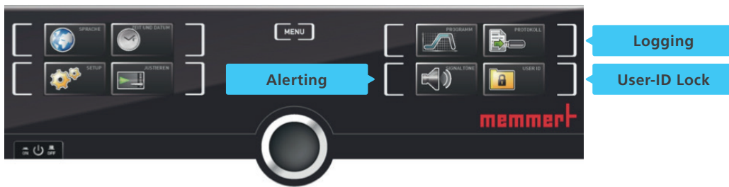
GMP-compliant functions of a climate chamber (©Memmert)
