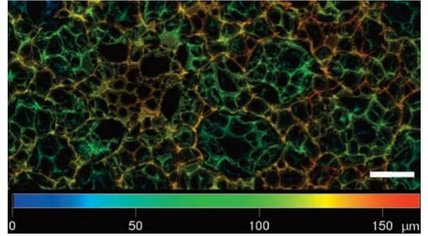
**Figure 9.** Depth colour-coded Z stack of cell-free Alvetex® Scaffold stained with Nile Red. Picture taken on a Zeiss LSM 510 confocal microscope. Note the depth of the Z-stack exceeds 150µm. Scale bar 50µm.
