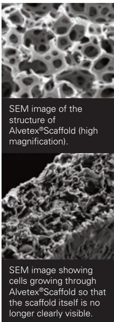
Alvetex® Scaffold is a 200µm thick highly porous, inert polystyrene scaffold that provides cultured cells with an optimal environment to grow in 3D. This allows for the formation of 3D niche microenvironments in which cell-cell interaction and communication networks occur.
