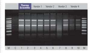
Pre-purified low concentration total RNA from human blood samples was concentrated using recommended protocols from different vendor kits. Purified RNA was analyzed on a 1% agarose gel. M – Thermo Scientific RiboRuler High Range RNA Ladder (#SM1821), C – RNA sample before concentration.
